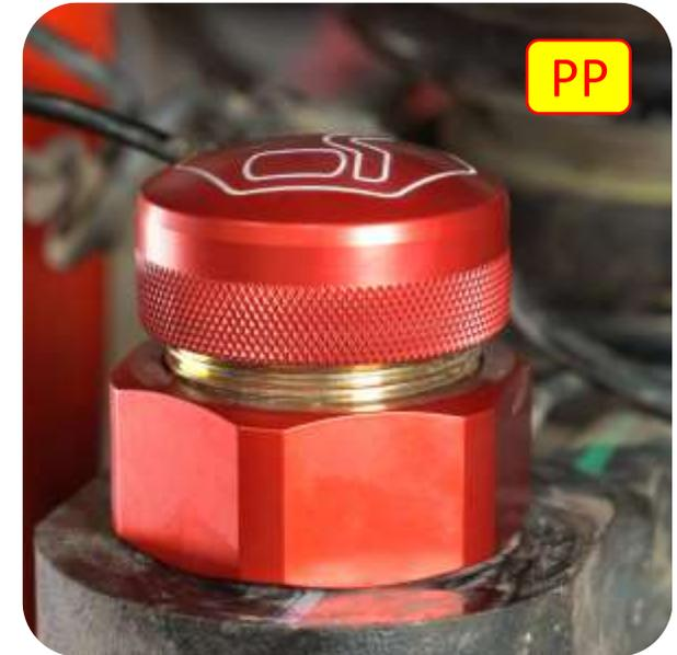
**Important Note:** *It is very important not to over tighten the assembly as this can cause a “Sticky” feeling in the steering and not return to center easily. If this condition exists after install, we recommend backing off the upper ball joint tensioner nut until loose and bringing just back into contact where resistance is felt in the wrench as tightening.*
