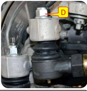
**Important Note:** The drag link nylock nuts that are included are a one time use ONLY; they should be replaced with a new one if removed.
