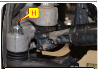
**Important Note:** The tie rod nylock nuts that are included are a one time use ONLY; they should be replaced with a new one if removed.
