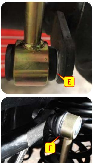
**Important Note:** *MetalCloak recommends using red Loctite on each of the upper spindles of the sway bar end links.*
