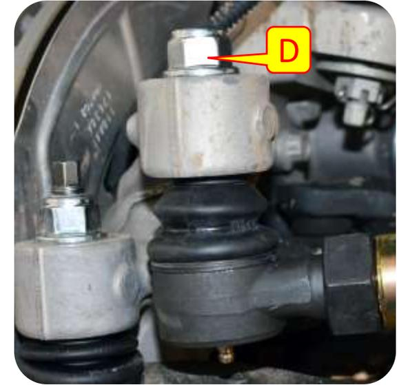
**Important Note:** The drag link nylock nuts that are included are a one time use ONLY; they should be replaced with a new one if removed.
